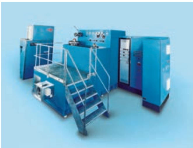
Test rig to determine pressure drop
