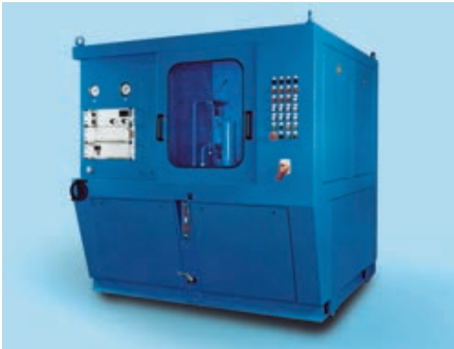
Collapse / burst pressure test rig
